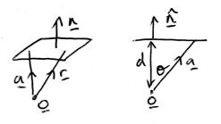
Here *d* is the perpendicular scalar distance of the plane from the origin, and  $\hat{n}$  is the unit normal. From the right-angled triangle we see that  $d = |a| \cos \theta = a \cdot \hat{n}$ . Thus an alternative form for the equation of the plane is  $r \cdot \hat{n} = d$ .
